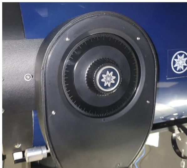
Figure 14: The dial in the center of the arm is the locking mechanism for the tube of the telescope.
