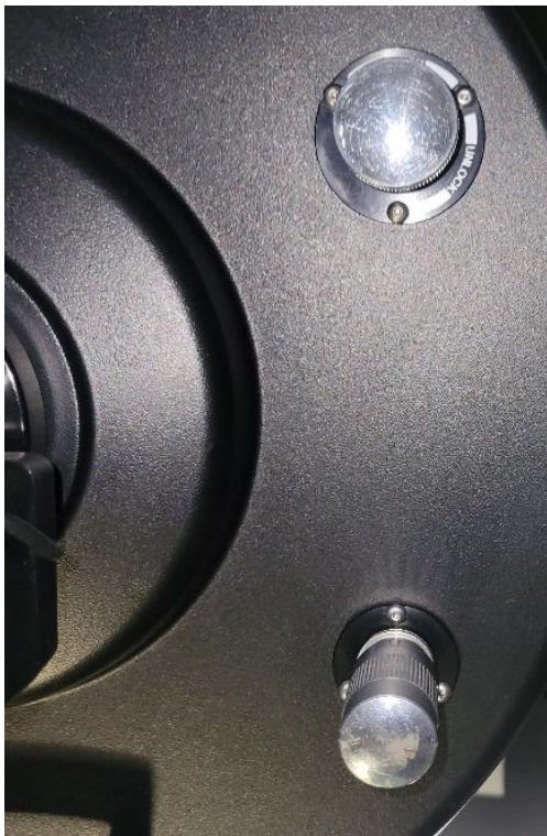
Figure 15: Pictured above are the 2 dials used to adjust the focus of the primary mirror inside the telescope.
