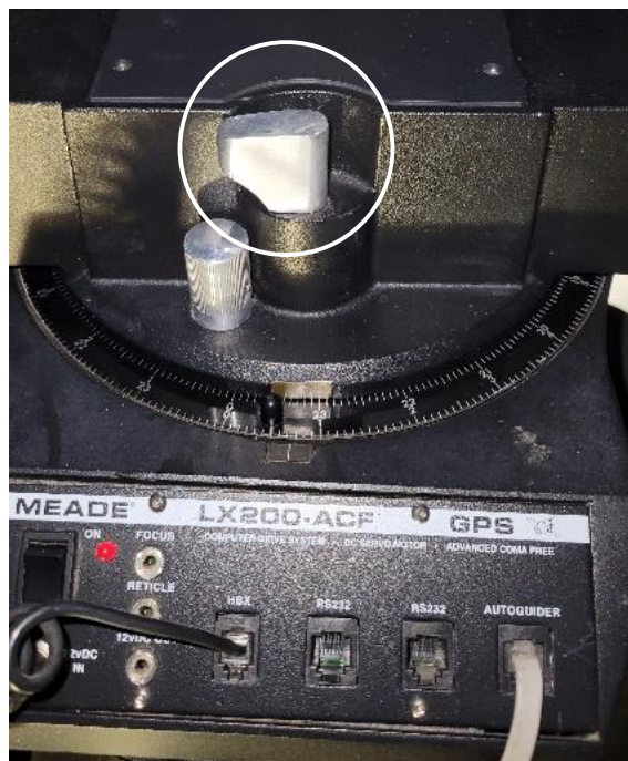
Figure 13: The flat silver piece, circled, in the center is the locking mechanism for the bottom gear of the telescope. When that lever is to the left the gear is locked and when it is flipped to the right the gear is free.
